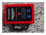
Once the selected Sealer has been applied readings with a slip meter shall be taken to confirm the finish floor surface is slip resistant when wet. This is defined as having a surface that gets a Co-efficient of Friction (CoF) reading greater than 0.4 or a Slip resistant value (SRV) of 39 or greater.
