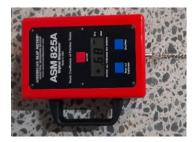
Once the selected Sealer has been applied readings with a slip meter shall be taken to confirm the finish floor surface is slip resistant when wet. This is defined as having a surface that gets a Co-efficient of Friction (CoF) reading greater than 0.4 or a Slip resistant value (SRV) of 39 or greater.
