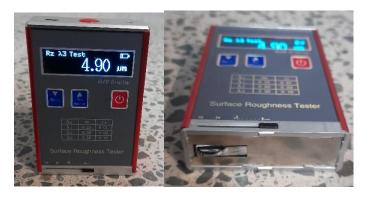
The Ra Meter measures both Metric and Imperial. The probe on the underside physically measures the texture of the surface to 0.00001mm. 1 micron= 0.001mm.
