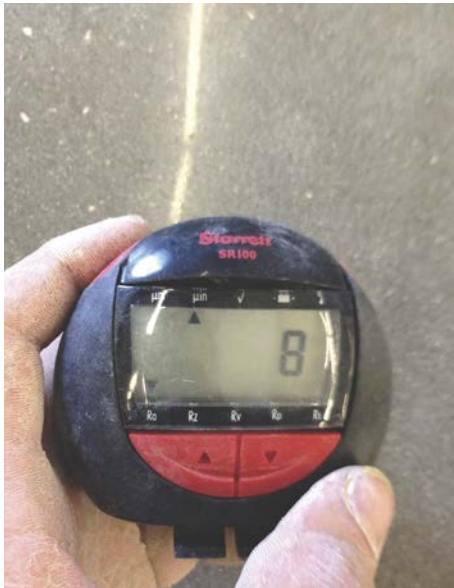
A surface roughness tester measures the texture of a polished concrete floor at 8 µin (microinches), an A-3 on the ST-115 Surface Texture Finishes Chart, equivalent to a 3,000-grit finish. Photo courtesy of Ardor Solutions.
